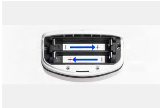
Figure 34 – Head Sensor with Battery Cover Removed
