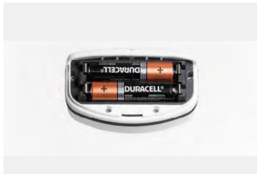
Figure 35 – Head Sensor with Batteries
