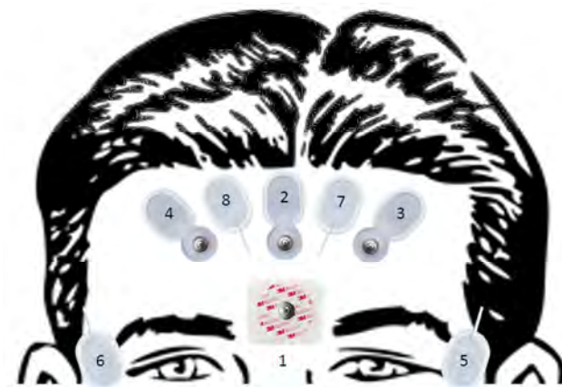
Figure 12 – Optimal 8 EEG Electrode Placement on Forehead
