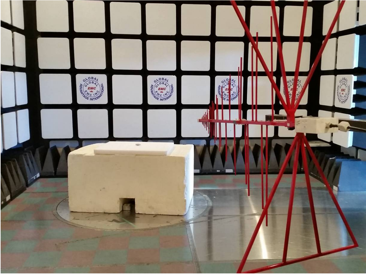
Figure 3 – Radiated Emissions Setup – Photo 2
