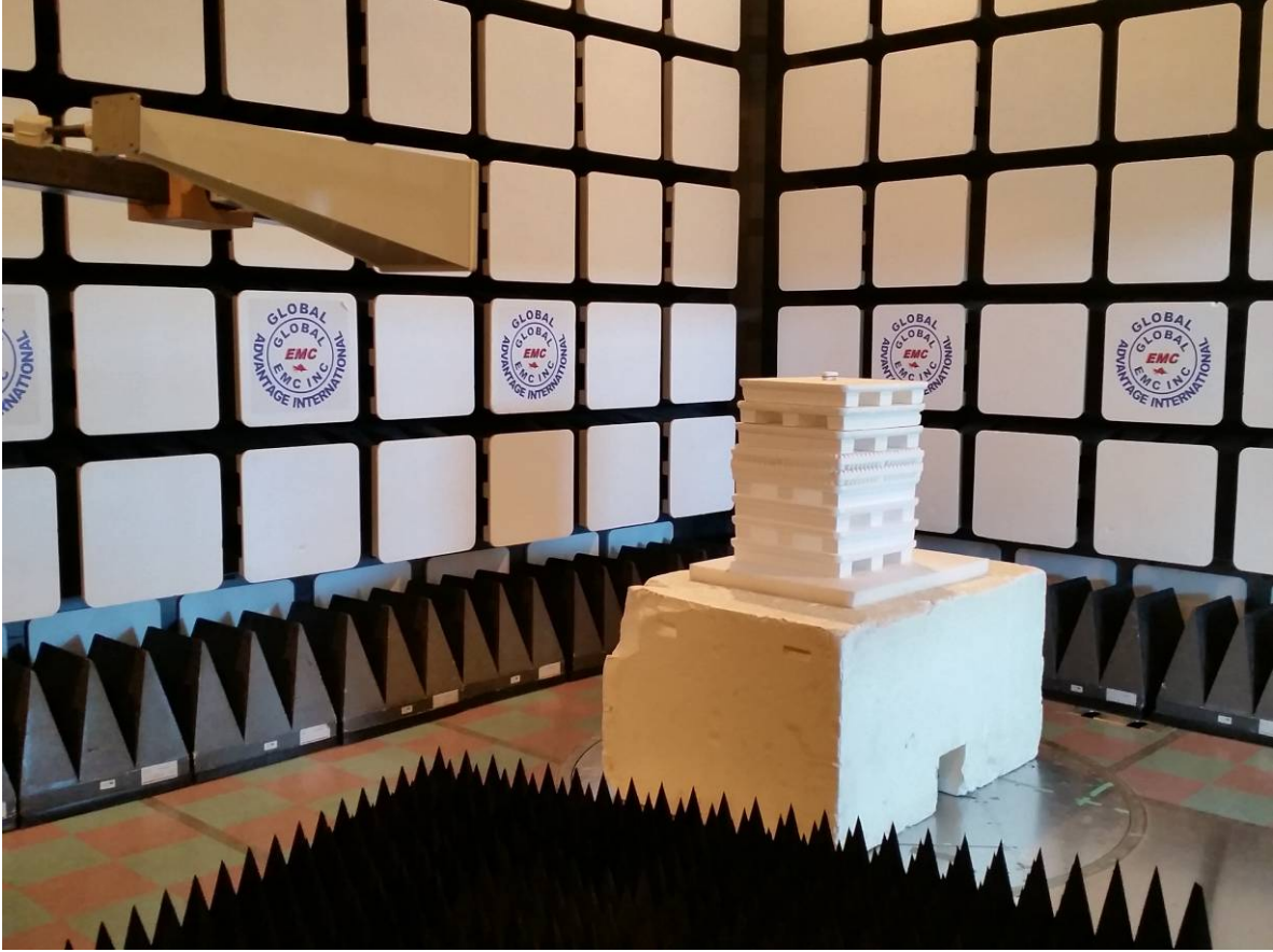
Figure 4 – Radiated Emissions Setup – Photo 3
