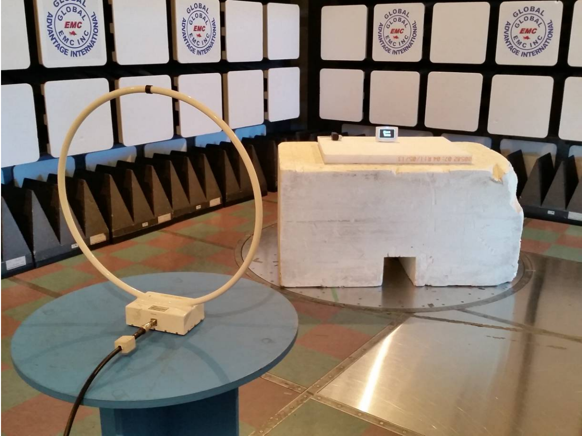
Figure 2 – Radiated Emissions Setup – Photo 1
