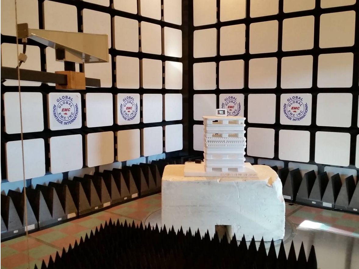
Figure 4 – Radiated Emissions Setup – Photo 3
