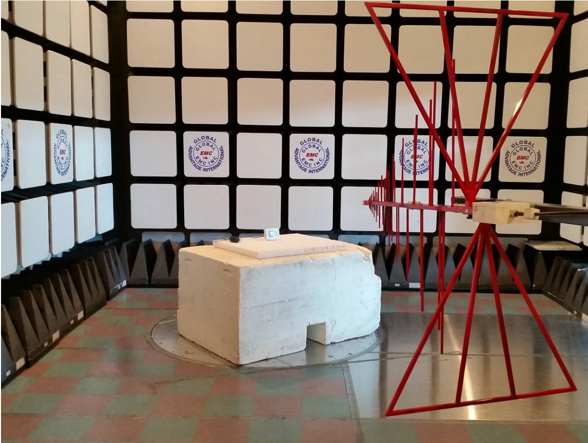
Figure 3 – Radiated Emissions Setup – Photo 2
