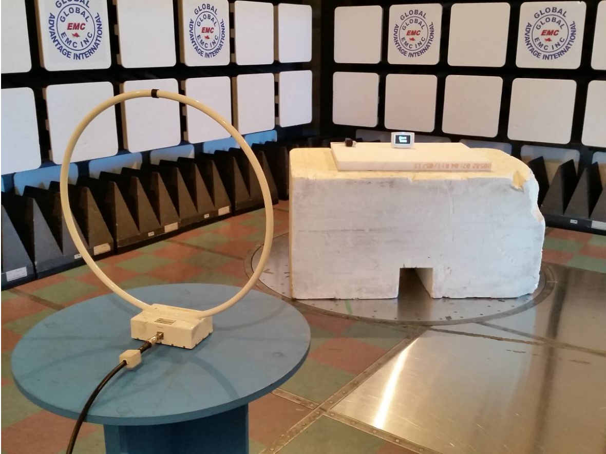
Figure 1 – Radiated Emissions Setup – Photo 1
