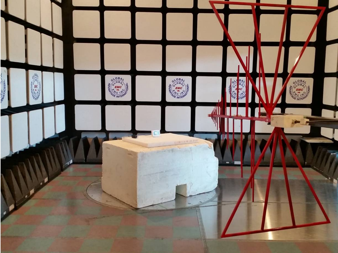
Figure 2 – Radiated Emissions Setup – Photo 2
