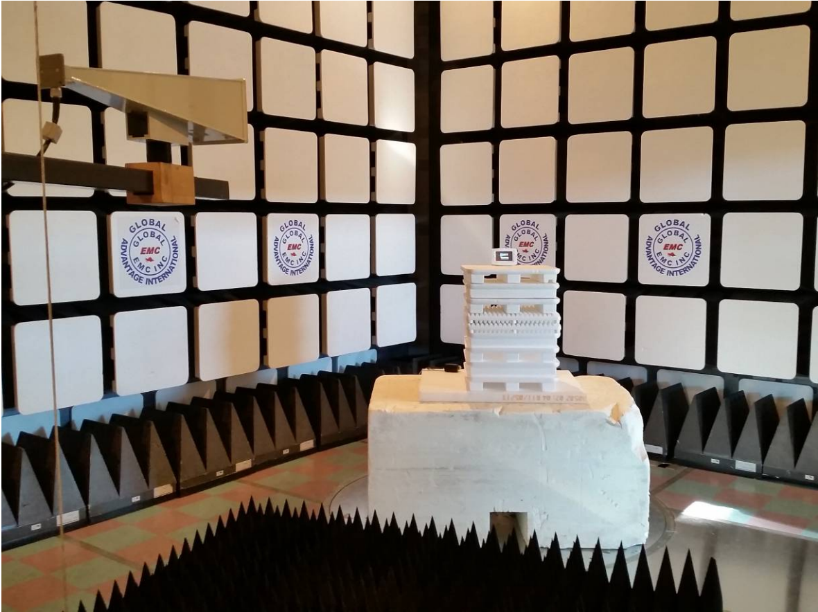
Figure 3 – Radiated Emissions Setup – Photo 3
