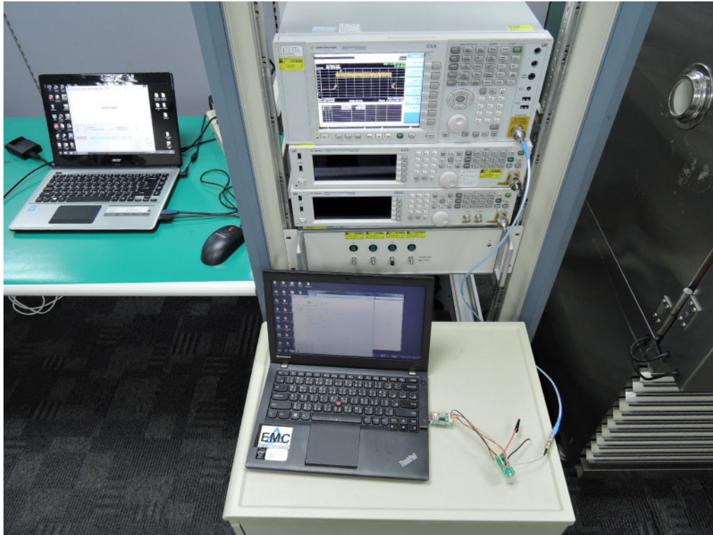
Photograph 4: Set-up for Conducted testing
