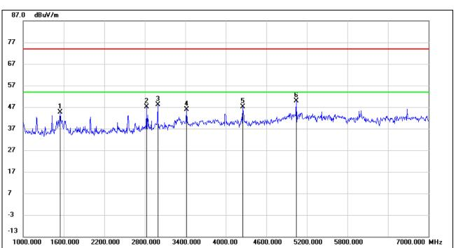
Remark Frequency Reading Correct Result Limit Margin No. (dB/m) (dBuV/m) (dBuV/m) (MHz) (dBuV) (dB) 1 1546.000 56.69 -11.99 44.70 74.00 -29.30 peak 2 2830.000 53.98 -6.81 47.17 74.00 -26.83 peak 3 2992.000 54.22 -6.10 48.12 74.00 -25.88 peak 4 3418.000 51.26 -5.37 45.89 74.00 -28.11 peak 5 4252.000 49.01 -1.84 47.17 74.00 -26.83 peak 6 5044.000 48.68 1.09 49.77 74.00 -24.23 peak
