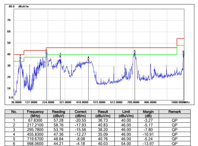
Note: 1. Result Level = Read Level + Antenna Factor + Cable loss.
