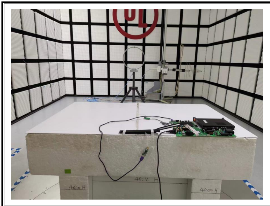
RADIATED RF MEASUREMENT SETUP (Below 30MHz)
