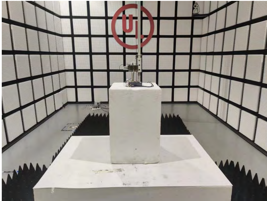
Radiated Disturbance Setup (Above 1 GHz – Worst Case)
