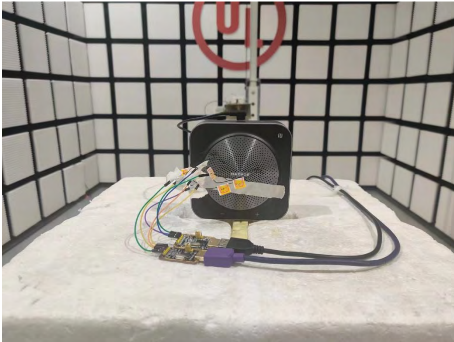
Radiated Disturbance Setup (Above 1 GHz – Z axis)
