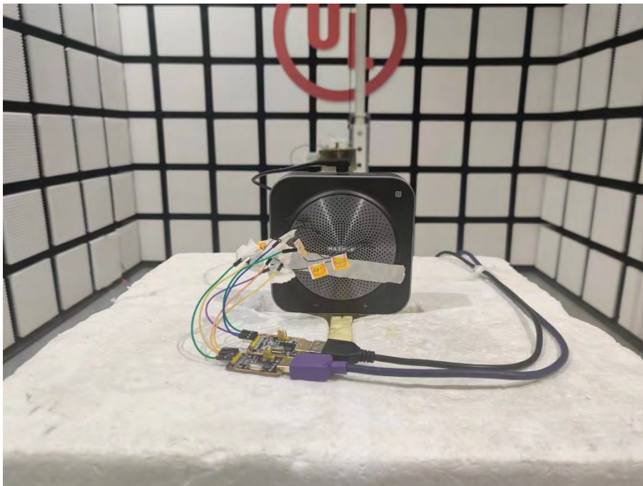
Radiated Disturbance Setup (Above 1 GHz – Z axis)
