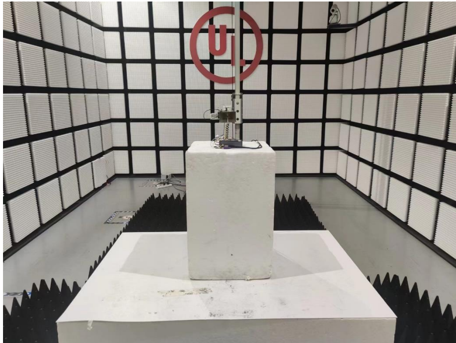
Radiated Disturbance Setup (Above 1 GHz – Worst Case)
