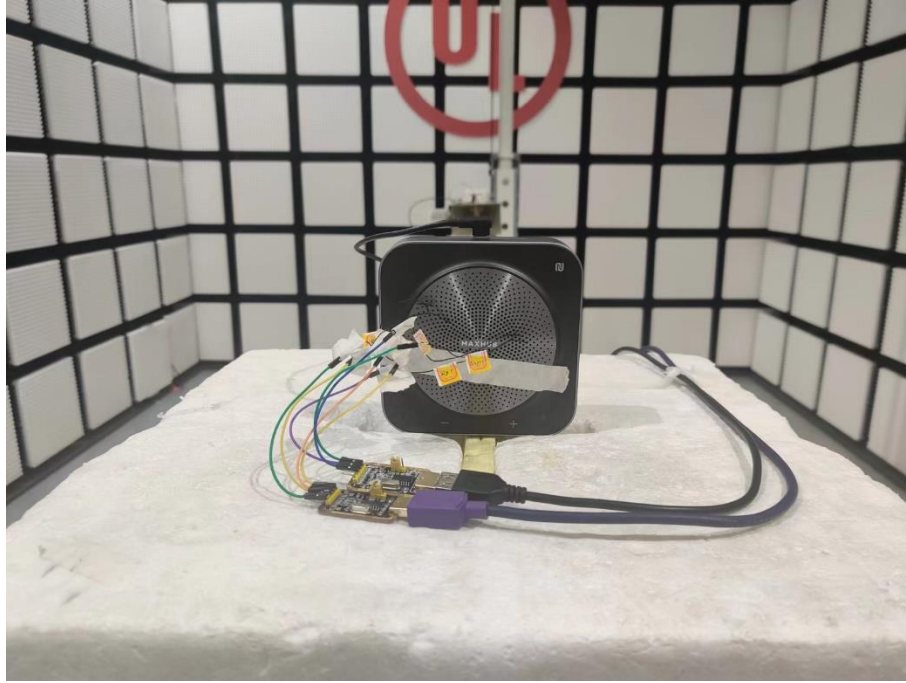
Radiated Disturbance Setup (Above 1 GHz – Worst Case)
