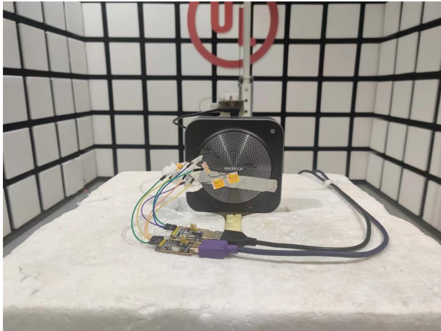
Radiated Disturbance Setup (Above 1 GHz – Z axis)
