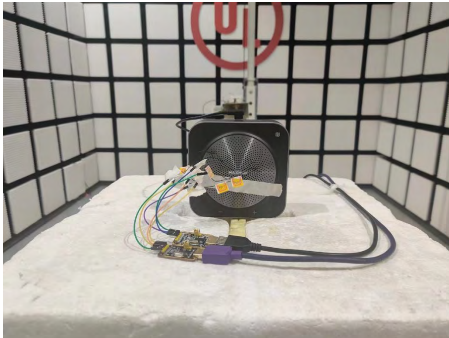
Radiated Disturbance Setup (Above 1 GHz – Z axis)
