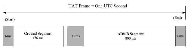
In this diagram, the ADS-B Segment is the only segment used for transmission by the ping2020 device. The start period in this segment is randomly assigned according to the UAT media access algorithm and the worst case duty cycle is derived from the last possible transmission time in the ADS-B segment back to back with the earliest possible transmission time in the next ADS-B segment. This gives a minimum period of 200mS between transmissions with the average period being much longer.
