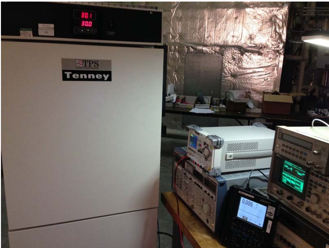
Frequency Stability, Chamber and Power Equipment
