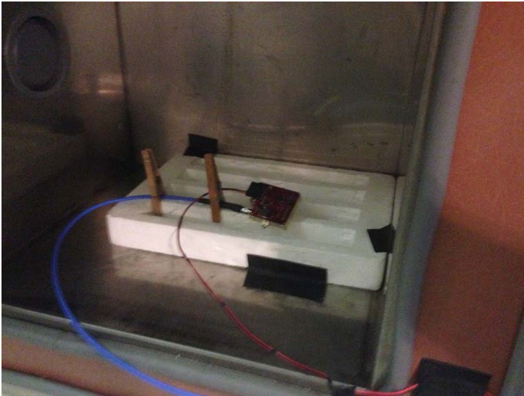
Frequency Stability, Chamber and EUT
