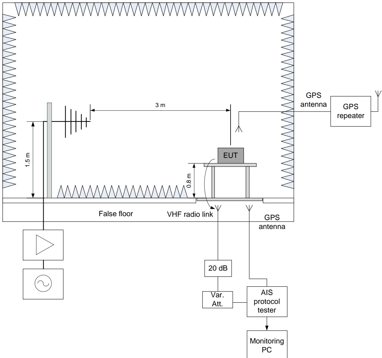
Monitoring of EUT: The output signals and correct timing were checked by using an AIS protocol tester.
