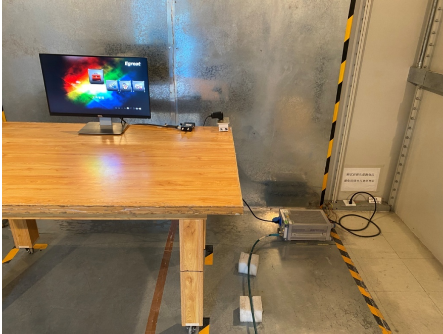
Conducted Emissions Side View
