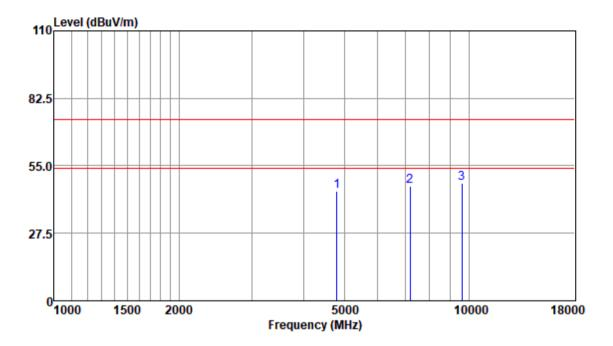
Test Mode: 00; Polarity: Vertical; Modulation:8DPSK; Channel:Low
