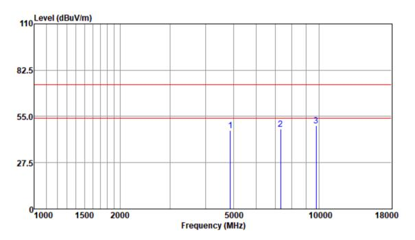
Test Mode: 00; Polarity: Horizontal; Modulation:8DPSK; Channel:middle
