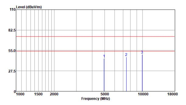
Test Mode: 00; Polarity: Horizontal; Modulation:GFSK; Channel:High
