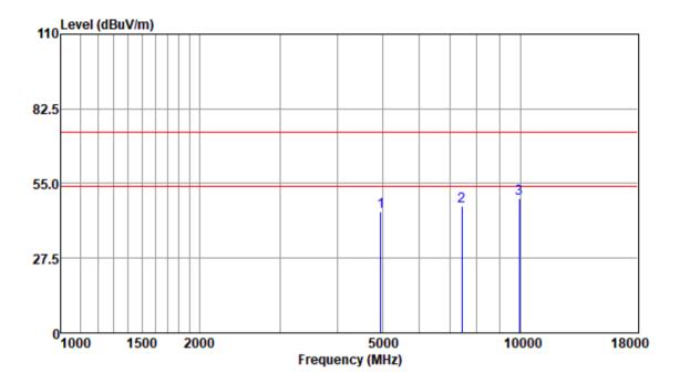
Test Mode: 00; Polarity: Vertical; Modulation:GFSK; Channel:High
