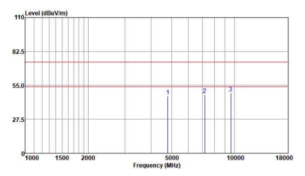
Test Mode: 00; Polarity: Horizontal; Modulation:8DPSK; Channel:Low
