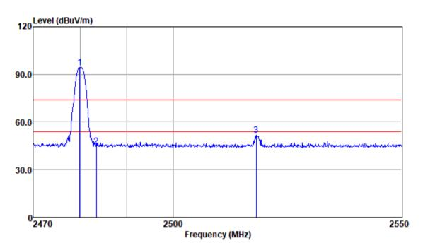
Test Mode: 00; Polarity: Horizontal; Modulation:8DPSK; Channel:High
