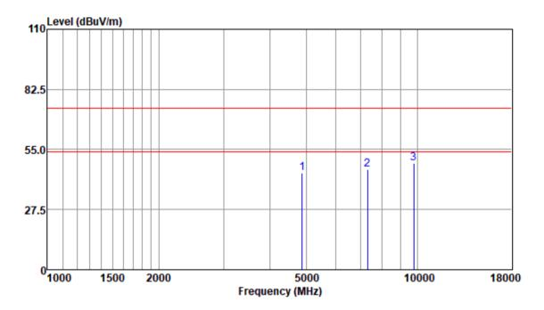
Test Mode: 00; Polarity: Vertical; Modulation:GFSK; Channel:middle
