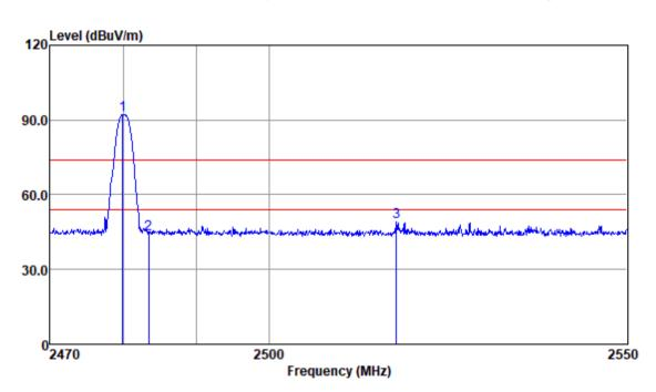
Test Mode: 00; Polarity: Vertical; Modulation:8DPSK; Channel:High
