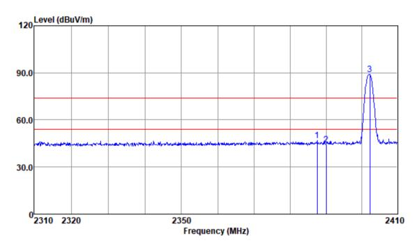
Test Mode: 00; Polarity: Vertical; Modulation:π/4 DQPSK; Channel:Low
