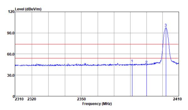
Test Mode: 00; Polarity: Horizontal; Modulation:8DPSK; Channel:Low
