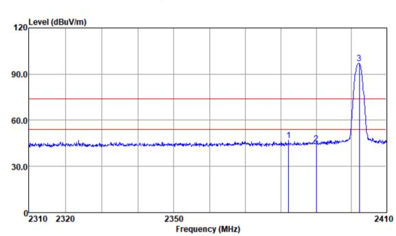
Test Mode: 00; Polarity: Horizontal; Modulation:GFSK; Channel:Low
