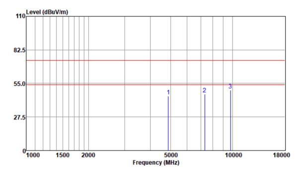
Test Mode: 00; Polarity: Horizontal; Modulation:GFSK; Channel:middle
