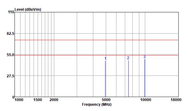
Test Mode: 00; Polarity: Vertical; Modulation:8DPSK; Channel:High
