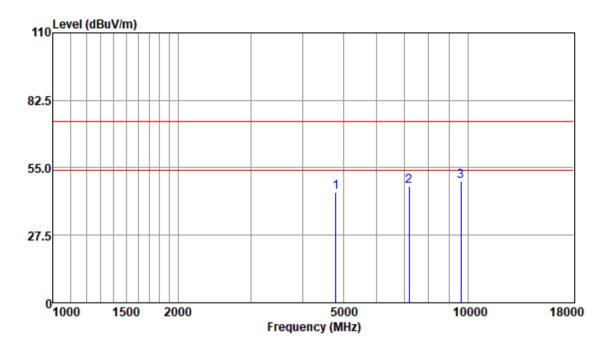
Test Mode: 00; Polarity: Vertical; Modulation:GFSK; Channel:Low
