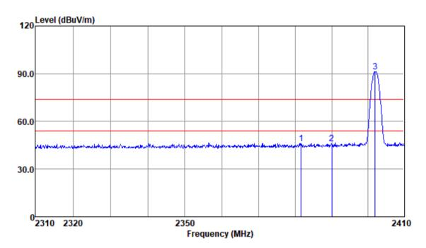
Test Mode: 00; Polarity: Vertical; Modulation:GFSK; Channel:Low
