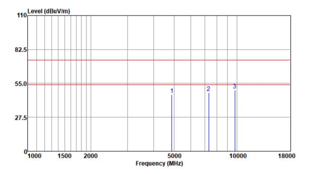
Test Mode: 00; Polarity: Vertical; Modulation:8DPSK; Channel:middle
