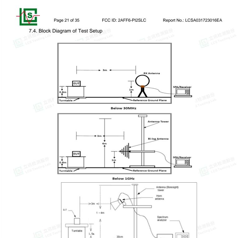
Above 1GHz Above 18 GHz shall be extrapolated to the specified distance using an extrapolation factor of 20 dB/decade form 3m to 1m.
