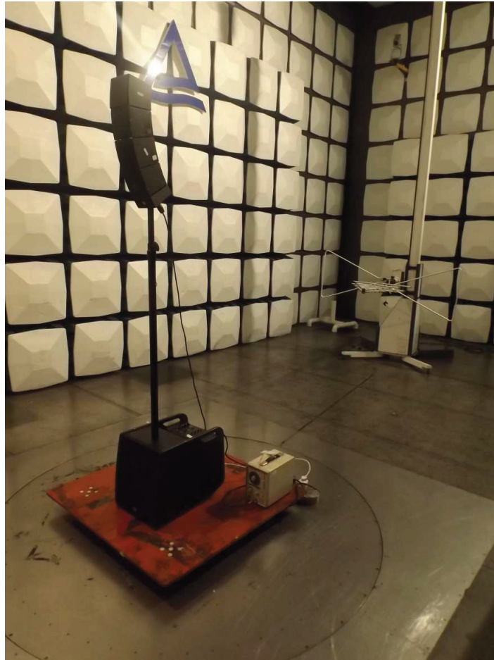
Photograph 2: Set-up for Spurious Emissions (30MHz-1GHz)
