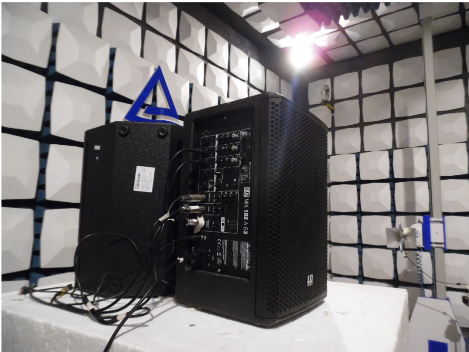
Photograph 2: Set-up for Spurious Emissions (above 1GHz)
