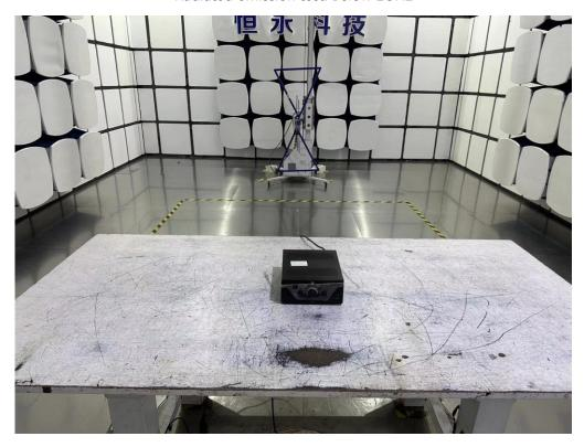
Radiated emission test: Above 1GHz
