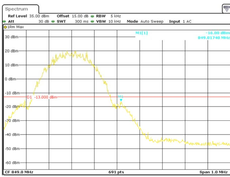
**PCS Band, Left Band Edge for GSM (GMSK) Mode**
