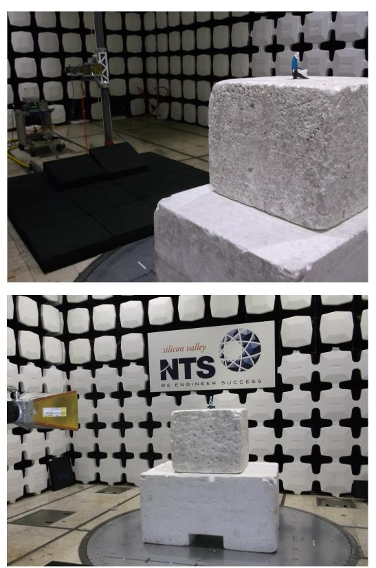
Radiated Emissions Test Configuration Photographs
