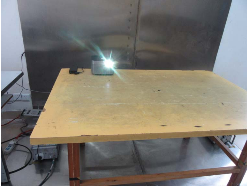
Conducted Emission Test Setup Front View
