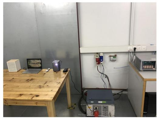
FCC RADIATED EMISSION TEST SETUP BELOW 1GHZ
