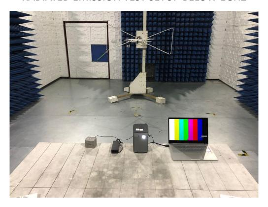
RADIATED EMISSION TEST SETUP ABOVE 1GHZ
