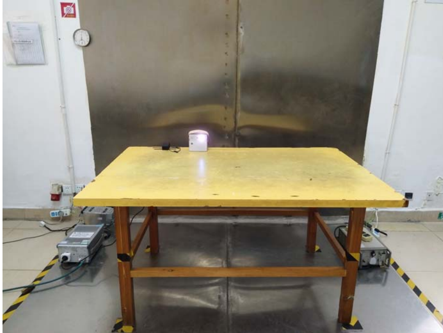
Conducted Emission Front View
