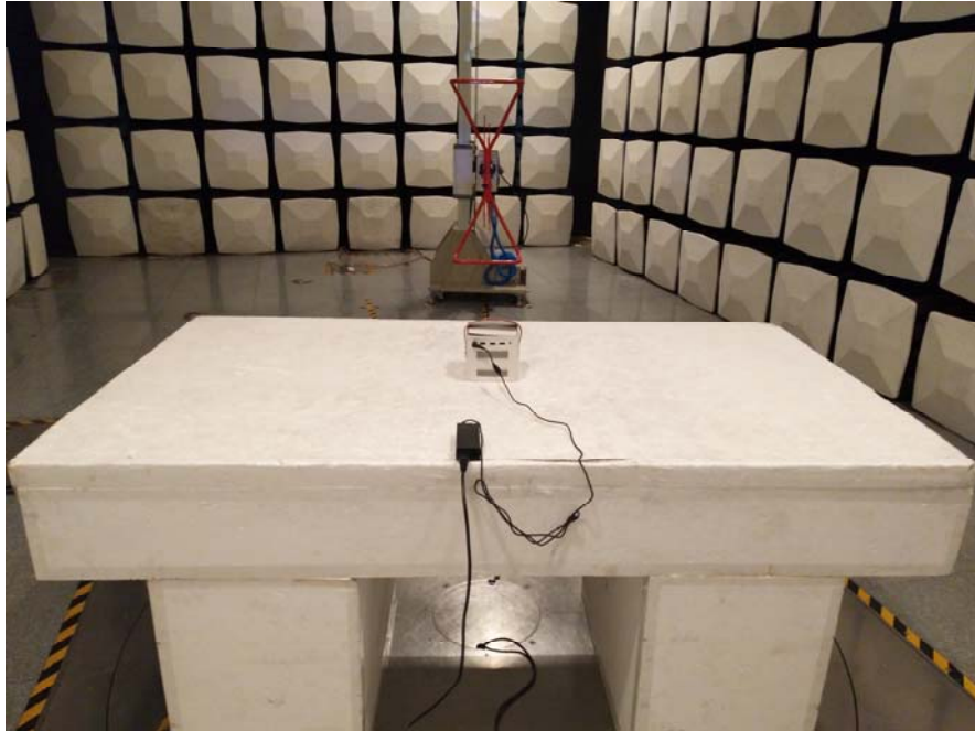
Radiated Emission View (Below 1 GHz)
