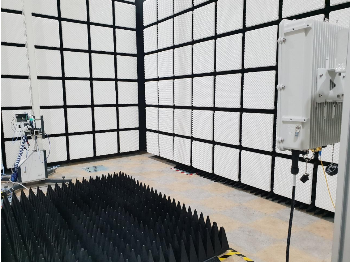
Radiated Test Setup Photo –Spurious (Horn Antenna 18 GHz ~ 40 GHz, Horizontal)
