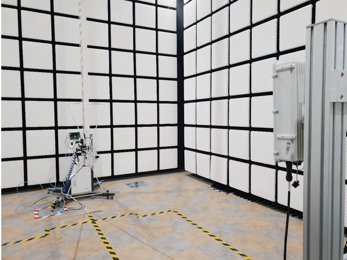
Radiated Test Setup Photo – Spurious (Bi-log Antenna, Vertical)
