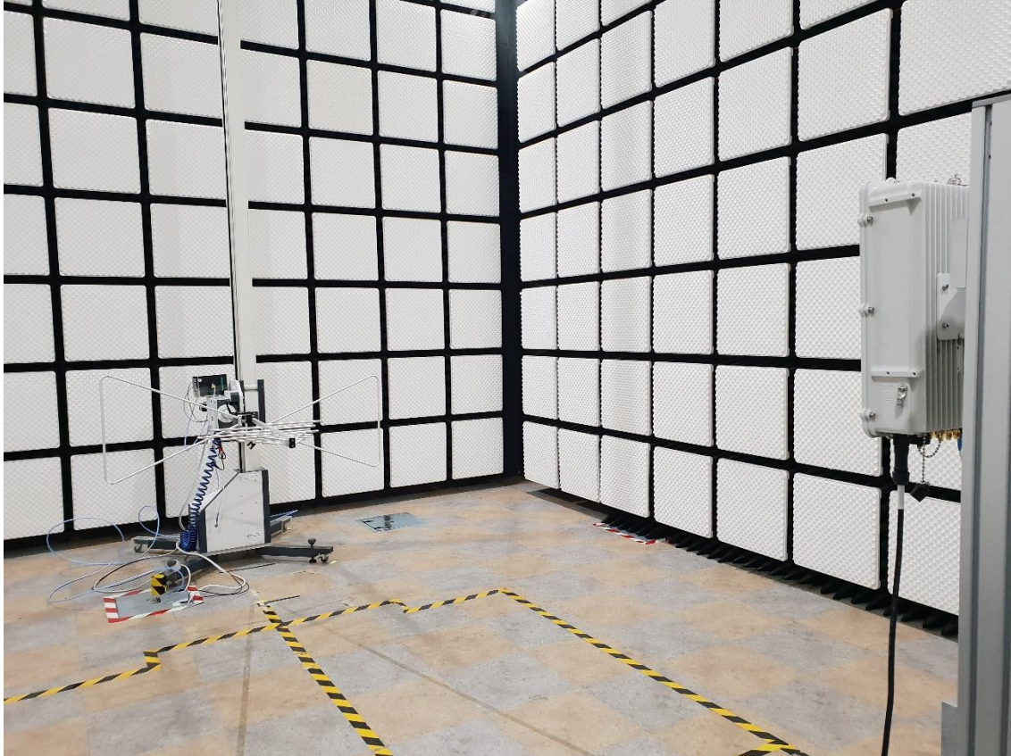
Radiated Test Setup Photo – Spurious (Bi-log Antenna, Horizontal)
