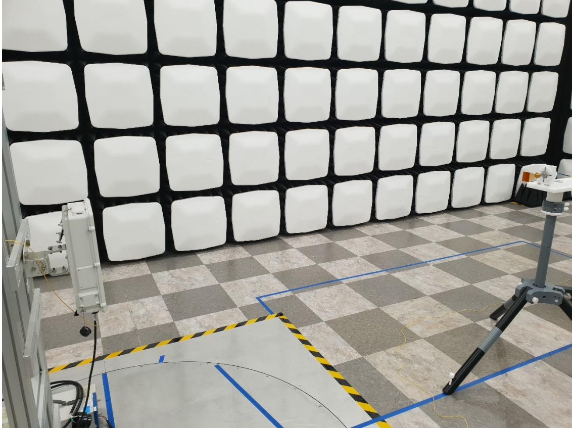
Radiated Test Setup Photo – Spurious (WR-19 Horn Antenna, Horizontal)
