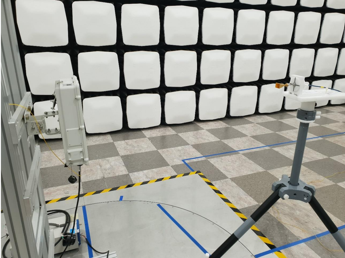
Radiated Test Setup Photo – Spurious (WR-12 Horn Antenna, Vertical)
