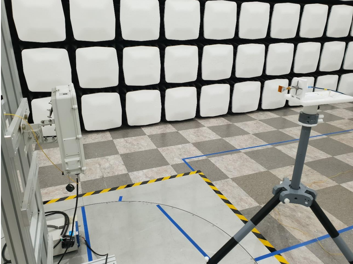
Radiated Test Setup Photo – Spurious (WR-12 Horn Antenna, Horizontal)
