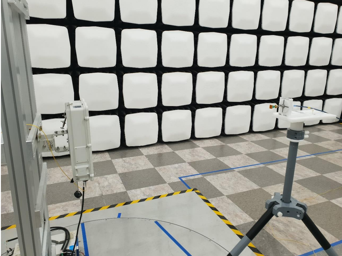
Radiated Test Setup Photo – Spurious (WR-08 Horn Antenna, Horizontal)
