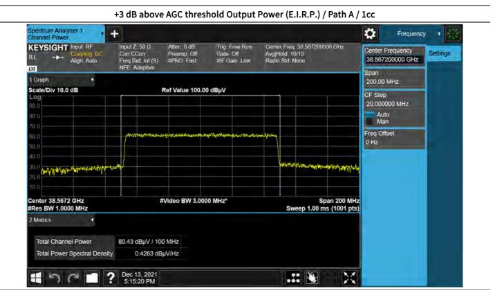
+3 dB above AGC threshold Output Power (E.I.R.P.) / Path A / 10cc
