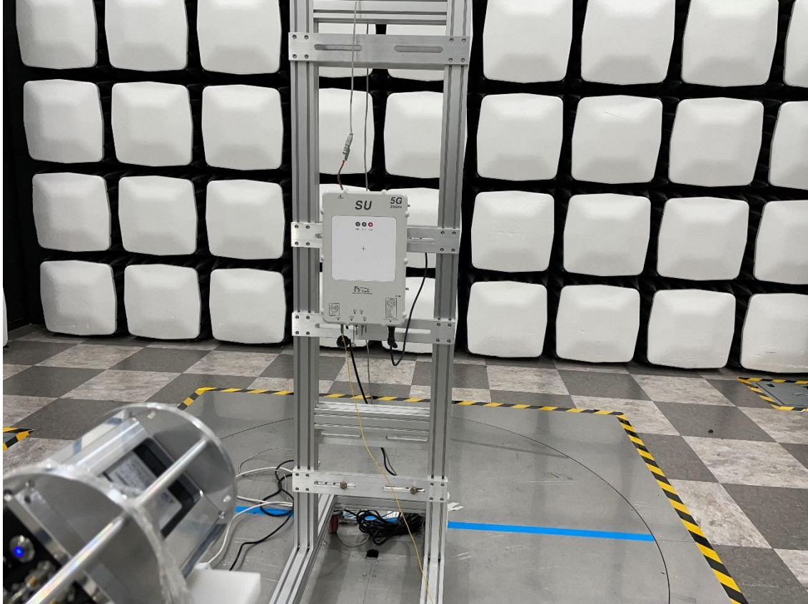
Radiated Test Setup Photo – Spurious (WR-05 Horn Antenna, 135°)
