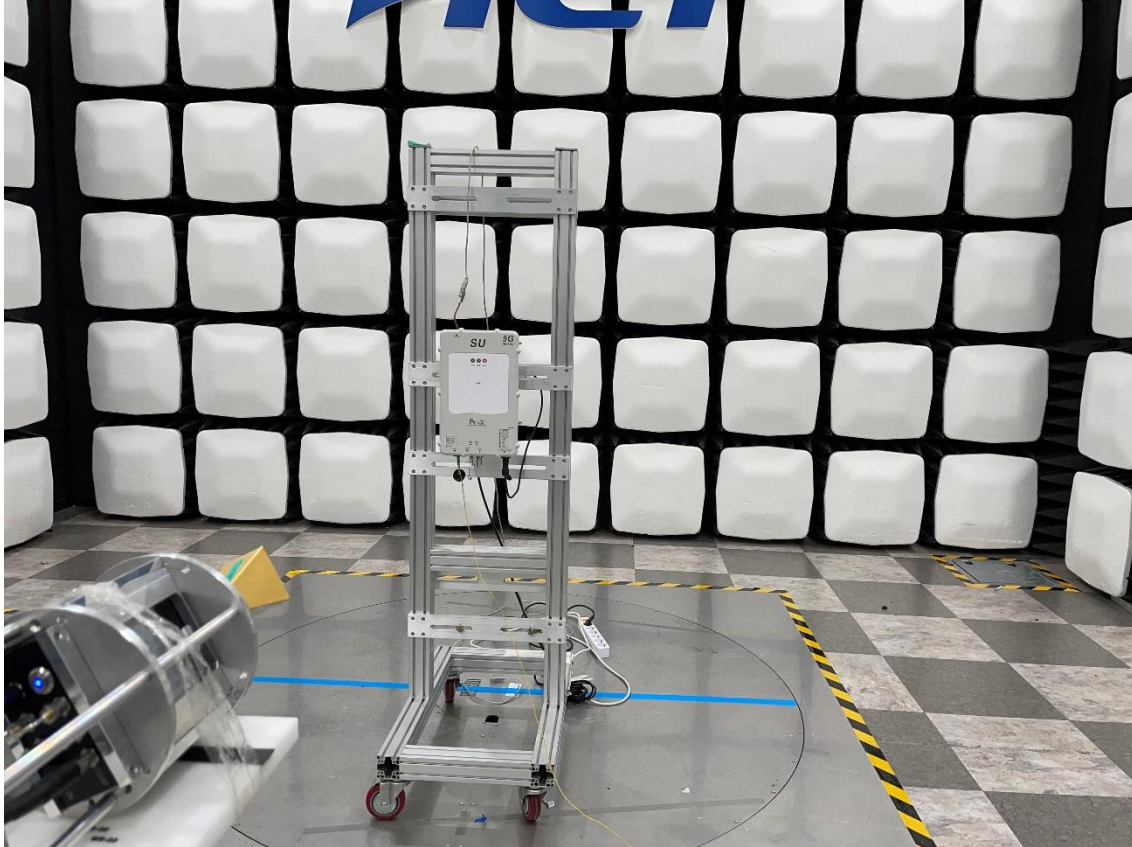
Radiated Test Setup Photo – Spurious (WR-19 Horn Antenna, 45°)
