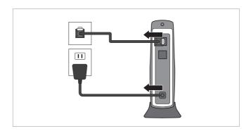
Connect one end of the supplied yellow RJ45 cable to the WAN port on the rear of ASRock X10 and the other end to the WAN port on your modem.
