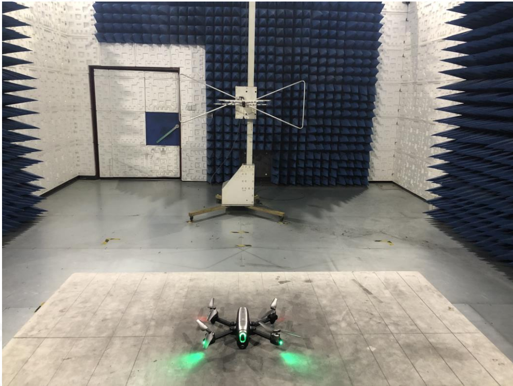
FCC RADIATED EMISSION TEST SETUP ABOVE 1GHZ
