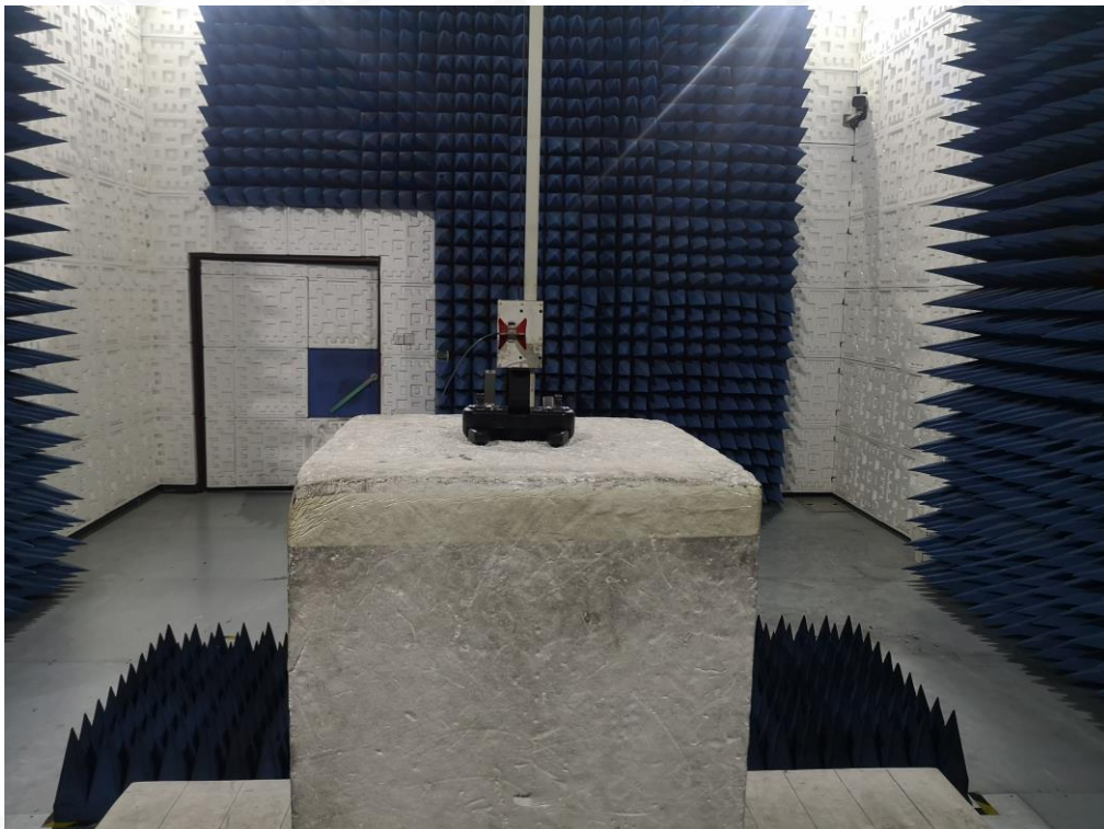
FCC RADIATED EMISSION TEST SETUP ABOVE 1GHZ
