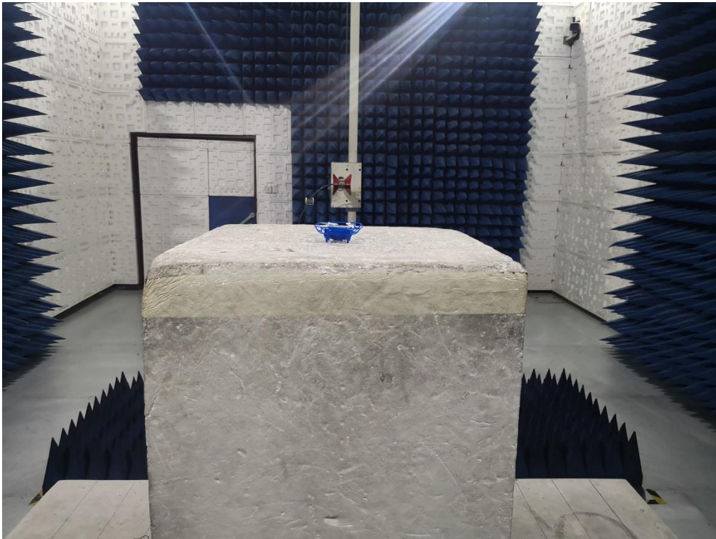
RADIATED EMISSION TEST SETUP ABOVE 1GHZ
