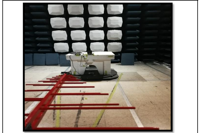
Figure R4: Radiated Emissions 30M-1G Test Setup
