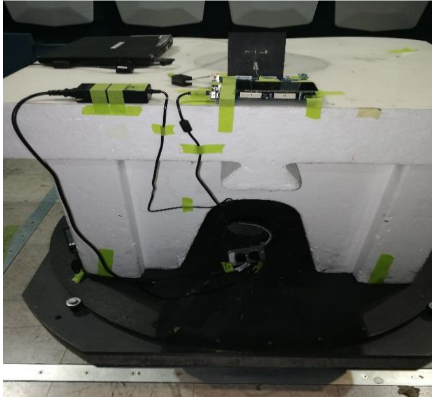
Figure R1: EUT Radiated Emissions Cable Layout
