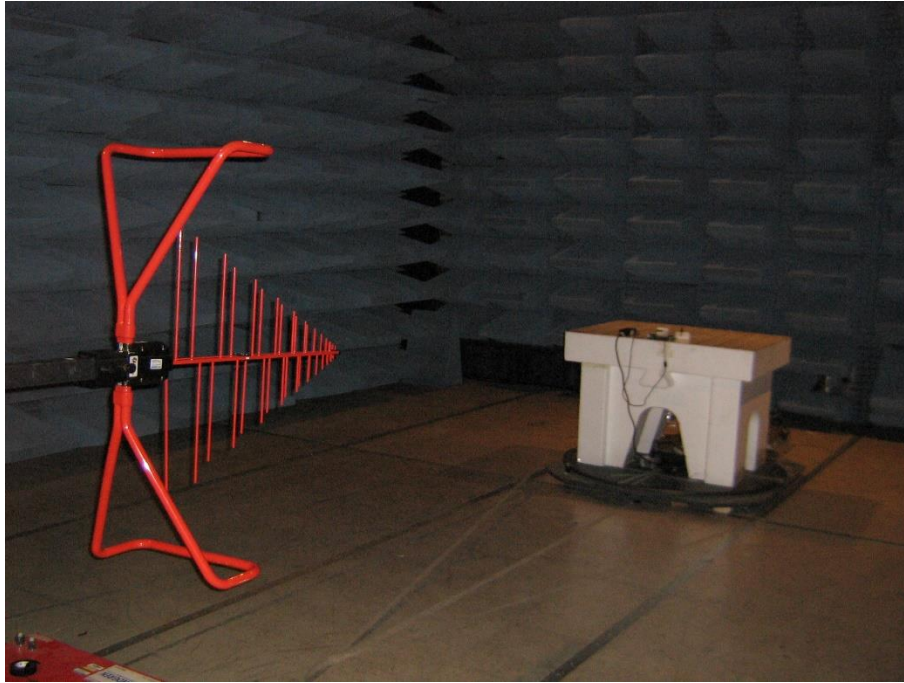
Radiated Emissions Test Setup - 30MHz-1GHz
