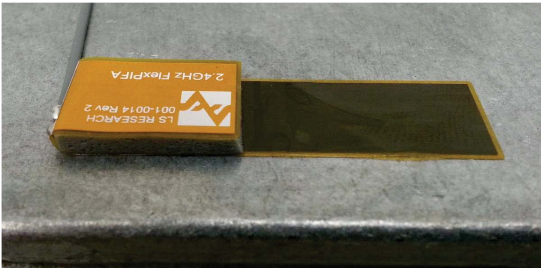
Figure 23 FlexPIFA Mounted on Metal
