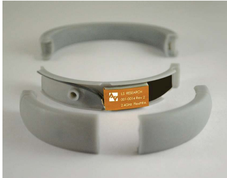
Figure 26 FlexPIFA Integrated into Bracelet
