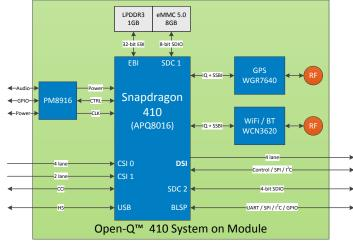
Deliver a superior user experience with the advanced quad-core ARM Cortex A53 CPU that is both 32bit and 64bit capable, the Hexagon DSP and Adreno 306 GPU. Includes support for OpenGL ES 3.0 and OpenCL
