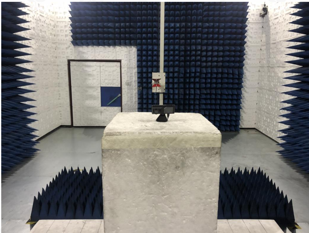
FCC RADIATED EMISSION TEST SETUP ABOVE 1GHZ
