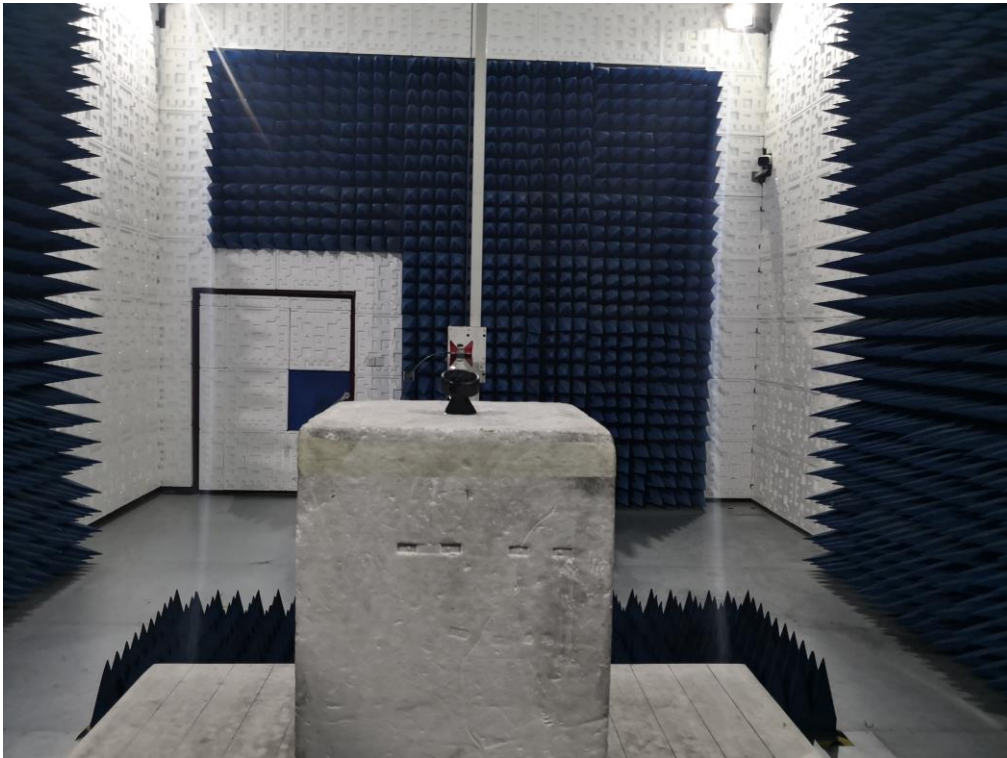
RADIATED EMISSION TEST SETUP ABOVE 1GHZ
