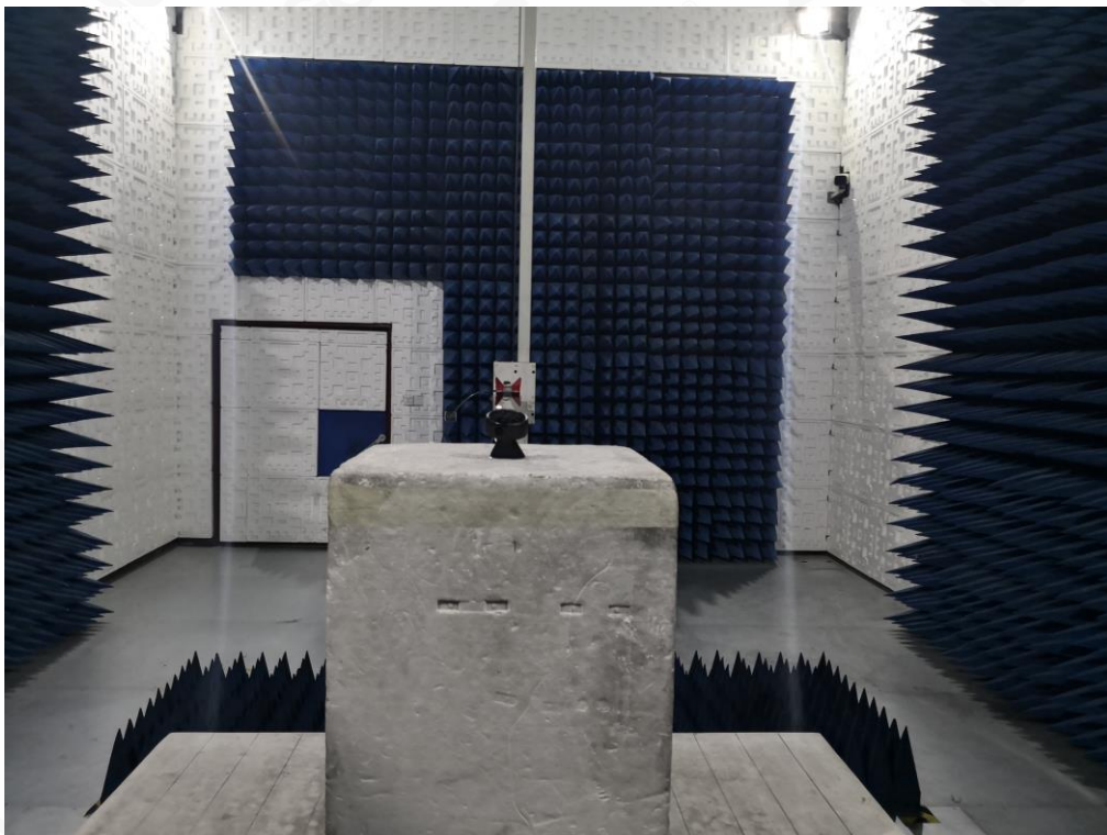
FCC RADIATED EMISSION TEST SETUP ABOVE 1GHZ
