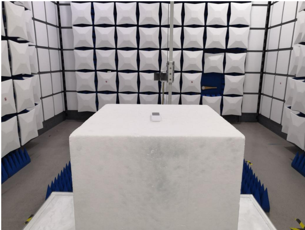
RADIATED EMISSION TEST SETUP ABOVE 1GHZ
