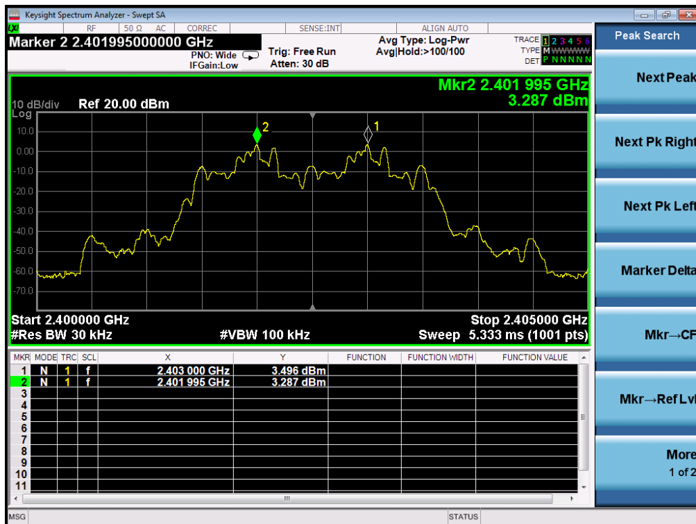
TEST PLOT FOR FREQUENCY SEPARATION
