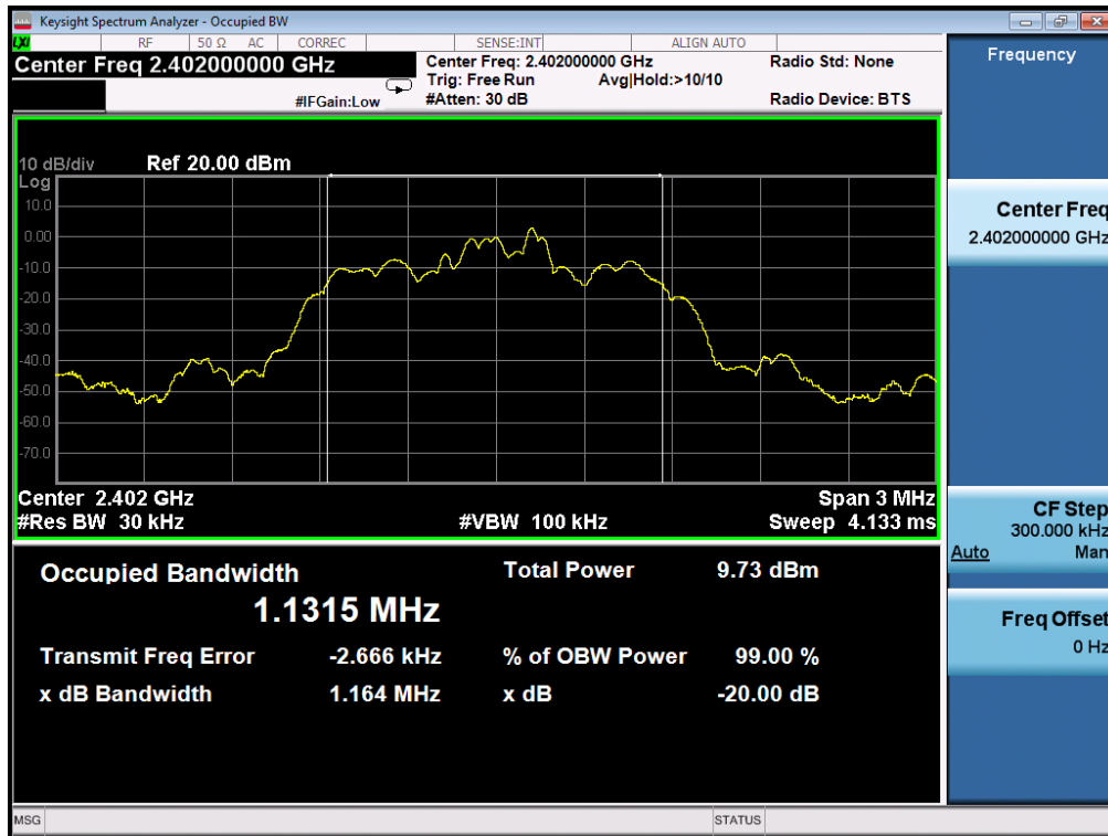
TEST PLOT OF BANDWIDTH FOR LOW CHANNEL
