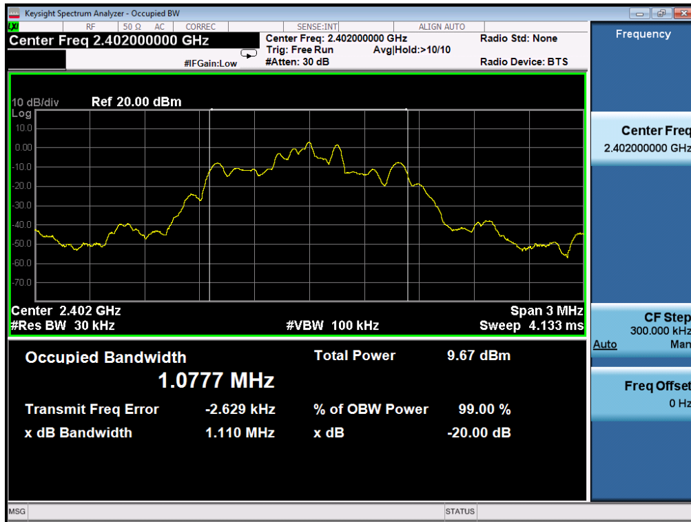
TEST PLOT OF BANDWIDTH FOR LOW CHANNEL
