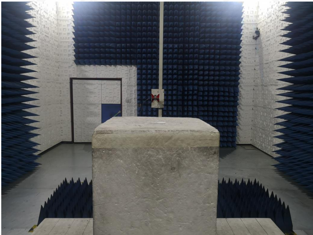
FCC RADIATED EMISSION TEST SETUP ABOVE 1GHZ
