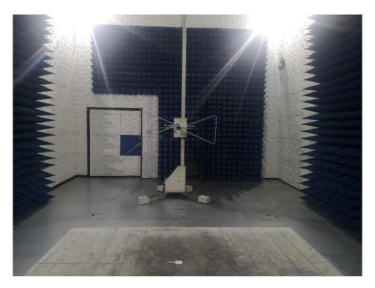
FCC RADIATED EMISSION TEST SETUP ABOVE 1GHZ
