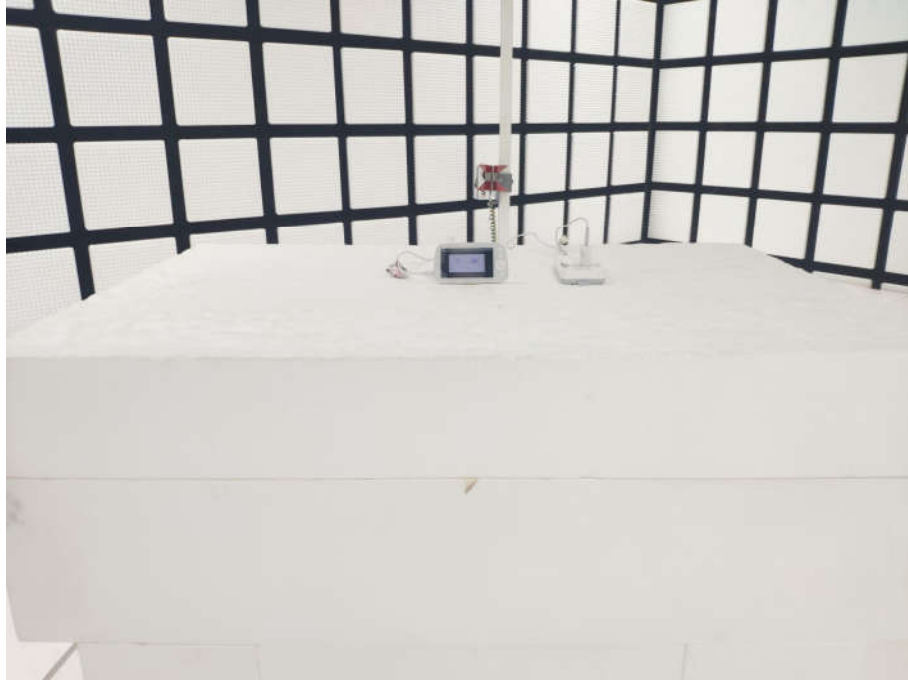
Radiated spurious emission Test Setup-3(Above 1GHz)
