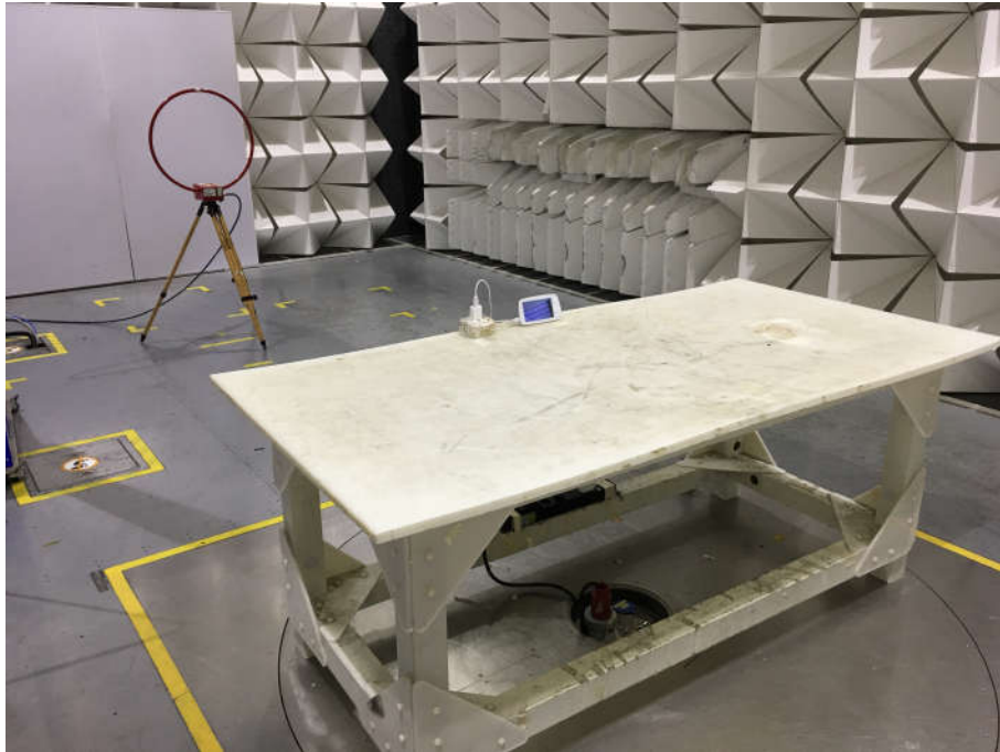
Radiated spurious emission Test Setup-1(Below 30MHz)
