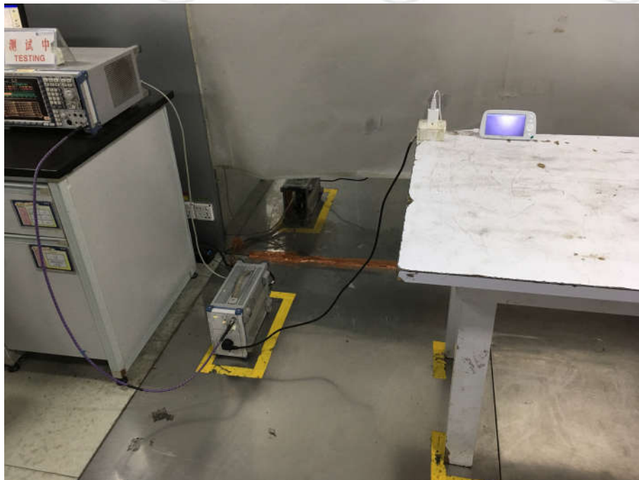
Conducted Emissions Test Setup
